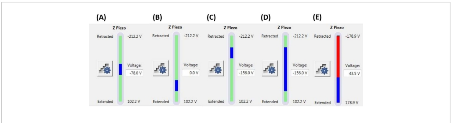
Figure 6: Ramp size and position. Z-piezo monitor showing the extent of the ramp (blue bar) relative to the total available Z-piezo movement range (green bar). (A) The Z-piezo position is near the middle of its range of movement, as indicated both by the blue bar being located roughly in the middle of the green bar and the current Z-piezo voltage (-78.0 V) being roughly between its fully retracted (-212.2 V) and extended (+102.2 V) values. (B) Z-piezo is extended relative to A , with no bias voltage applied. (C) Z-piezo is retracted relative to A and B . (D) The Z-piezo position is the same as in C at -156.0 V, but the ramp size has been increased relative to A-C to take advantage of more of the Z-piezo's full range of motion. (E) The ramp size is too large for the current ramp position, resulting in the Z-piezo being extended to the end of its range. This will cause the F-D curve to flatline as the system cannot extend the Z-piezo further. Abbreviation: F-D = force-displacement. Please click here to view a larger version of this figure.
